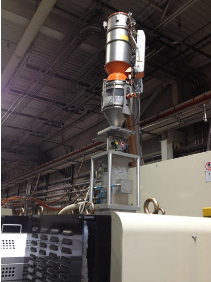
EXTRACTOR in the Combination with PROTECTOR for the protection of injection moulding machinery
