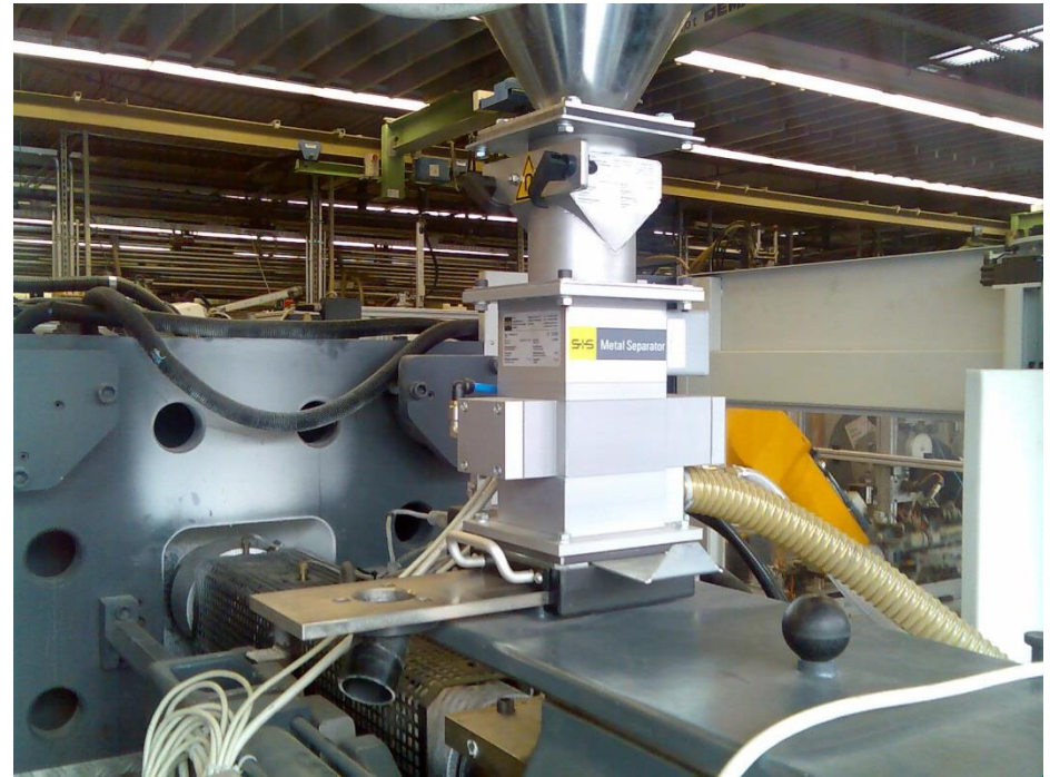
EXTRACTOR in the Combination with PROTECTOR for the protection of injection moulding machinery
